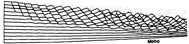
Fig. 7. Cartoon to show progressive crustal attenuation across a basin in which extension is accommodated at shallow levels by rotational block faulting and at deeper levels by flow (redrawn after Morton & Black 1975, and Chamberlain 1983). The stippled region represents post-stretching basin infill. Note how extension and tilt increase across the basin, and how internal deformation of the fault bounded blocks (particularly at depth) is able to take up differential tilting.
